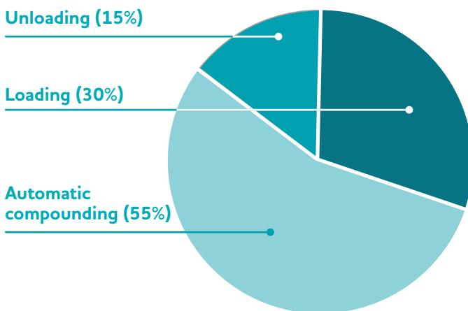
As presented in the **pie chart on the left**, the automatic compounding process accounted for an average of 55% of the cycle time, while the loading and unloading tasks accounted for an average of 30% and 15% of the cycle time respectively.
