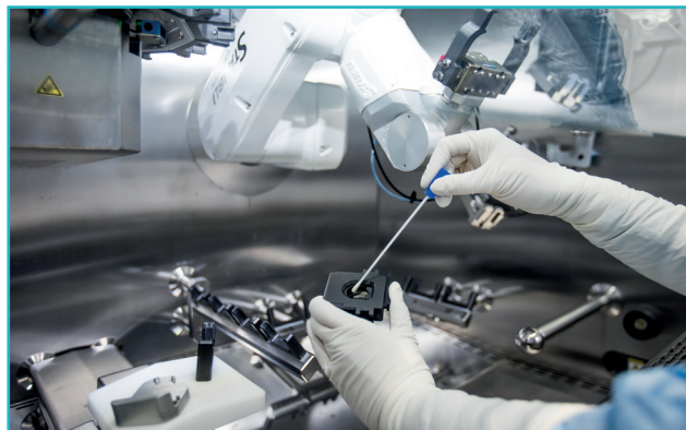
Figure 3. Swab sampling of irregular surfaces for measuring surface bioburden. Swabs were subsequently transferred to contact plates to recover bioburden.
