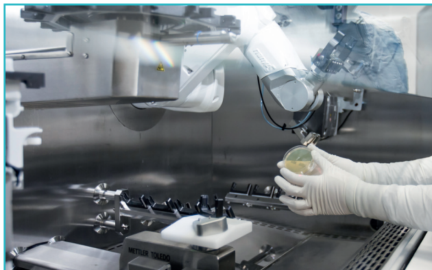
Figure 2. Contact plates for measuring surface bioburden.
